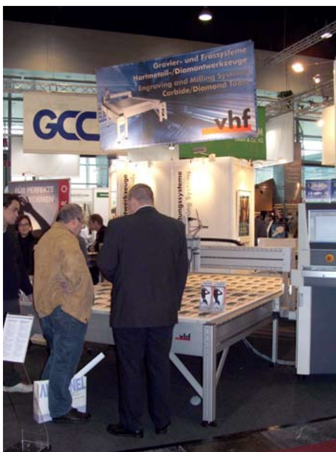
The large-scale milling and cutting system CAM 2030 Active Pro while cutting a printed plate with automatic register mark recognition
