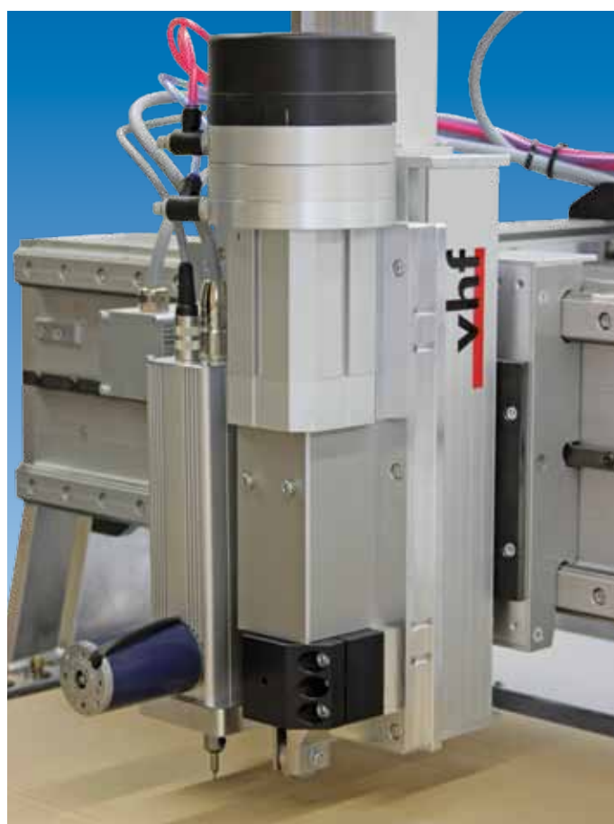
Folding device, here mounted to the right of an oscillating tangential cutting head.
