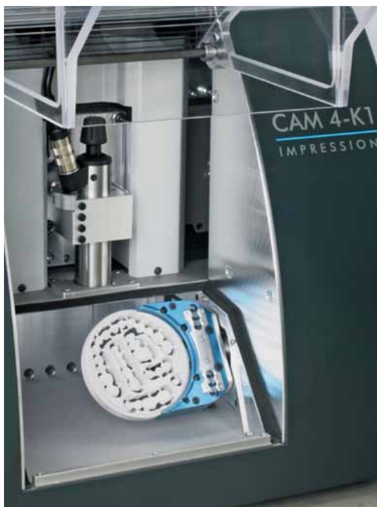
Detail view of the machining area of a CAM 4-K1 Impression: a high frequency spindle with quick chucking device and the highly precise Harmonic-Drive rotary axis with fixing device for universal blanks.
