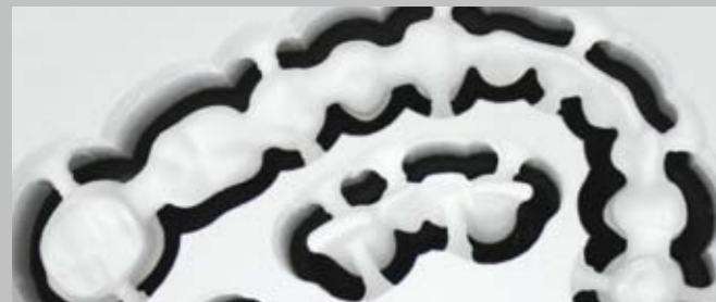
Detail view of the top of a zircon blank – you can mill bridge frameworks with up to fourteen units.
