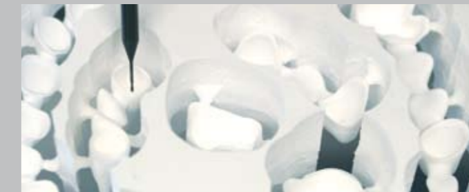
Detail view of the machining process at the bottom side of a zircon blank with a special dental radius milling cutter.
